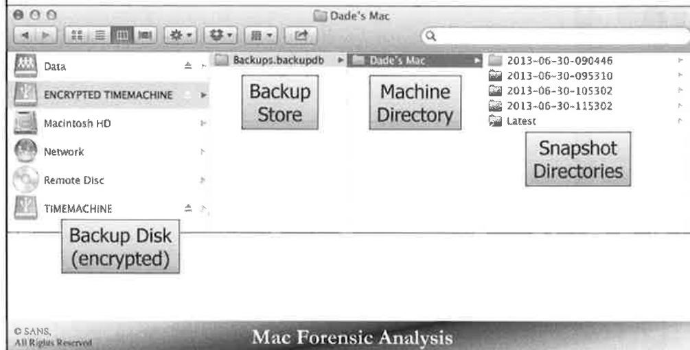
Once mounted, the encrypted backup volume follows the same basic structure as a non-encrypted external backup volume, including metadata.
