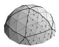
One of the ways Buckminster Fuller would describe the differences in strength between a rectangle and a triangle would be to apply pressure to both structures. The rectangle would fold up and be unstable but the triangle withstands the pressure and is much more rigid --- in fact the triangle is twice as strong. This principle directed his studies toward creating a new architectural design, the geodesic dome, based also upon his idea of
